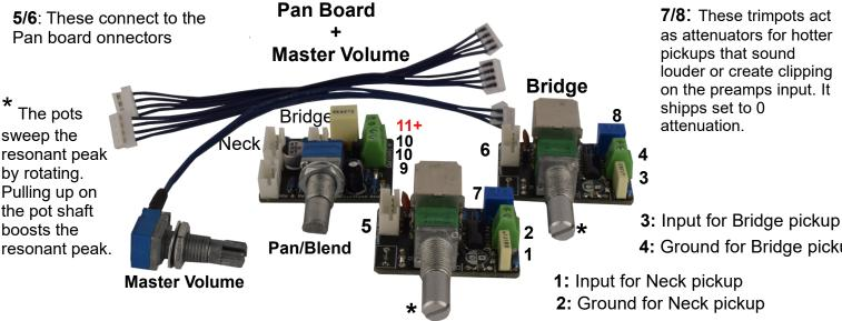
**7/8**: These trimpots act as attenuators for hotter pickups that sound louder or create clipping on the preamps input. It
