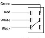
Finished Switch Wiring
