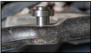
5. Place the Tapered Sleeve Adapter into the Drag link hole.
