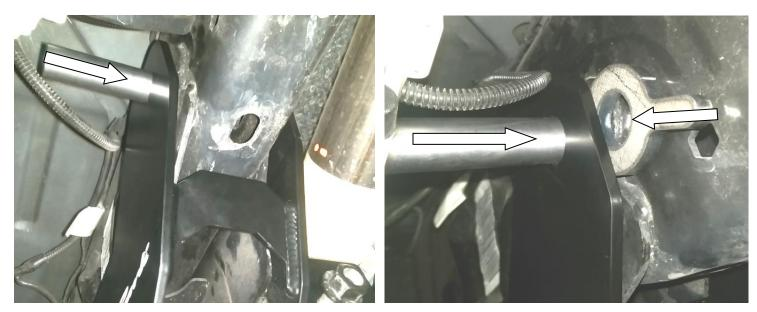
**13.** Install the 18MM x 1.5" bolts into the factory location using a washer on each side. The inside bolt should be installed first to ensure sufficient room for the ratchet in the drops. Torque to 280ft.lbs.
