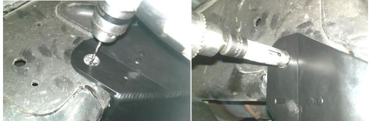
**18.** Slide the <sup>3</sup>/<sub>4</sub>" OD Crush Sleeve into the provided tool (L-Bracket). Once it's pressed in and centered, slide the <sup>3</sup>/<sub>4</sub>" crush sleeve into the upper, rear frame hole that you just drilled. The L-Bracket will index off the drop. With the tool inserted, clamp it in place to ensure it remains flat during drilling.
