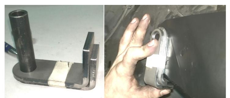
**19.** Use a ½" Drill bit to slide into the tool/indexed crush sleeve and drill the opposing side of the frame rail. **Note:** A right-angle drill will be necessary here.
