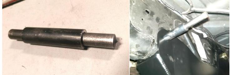
**17.** Remove the sleeve and punch and use a pilot bit to drill the center-punched hole. Then, use the provided <sup>3</sup>/<sub>4</sub>" hole saw to drill the frame to match the rear bracket hole.
