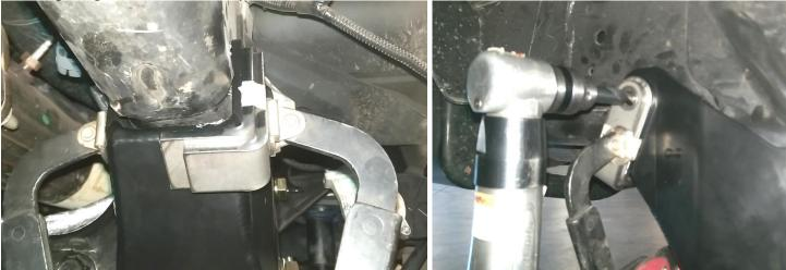
20. Once drilled, remove the crush sleeve and pull the L-Bracket indexing tool off of the <sup>3</sup>/<sub>4</sub>" OD Crush sleeve.
