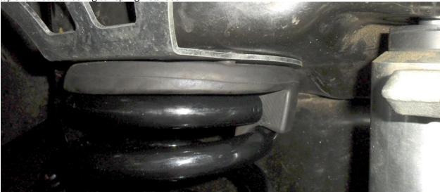
**6.** Compress the front suspension so the weight of the truck is on the spring and install Adjustable Carli Track Bar, Radius Arm Drop Brackets, Sway Bar Drop Brackets & Factory end links; then re-secure the driveshaft & brake line brackets to the axle and install your Carli Front Shocks..
