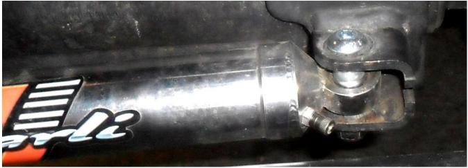
8. Adjust the stabilizer to desired pressure within operating range of 70-200psi as stated in "Special Notes Adjustment: Carli Stabilizers come pre-charged with 200PSI of Nitrogen. If a right-hand pull is encountered after installation, Nitrogen pressure should be released to reduce the stabilizer push by depressing the Schrader for a fraction of a second. RELEASE AS LITTLE AS POSSIBLE. Drive the truck and repeat if necessary. DO NOT run stabilizer with less than 70PSI!
