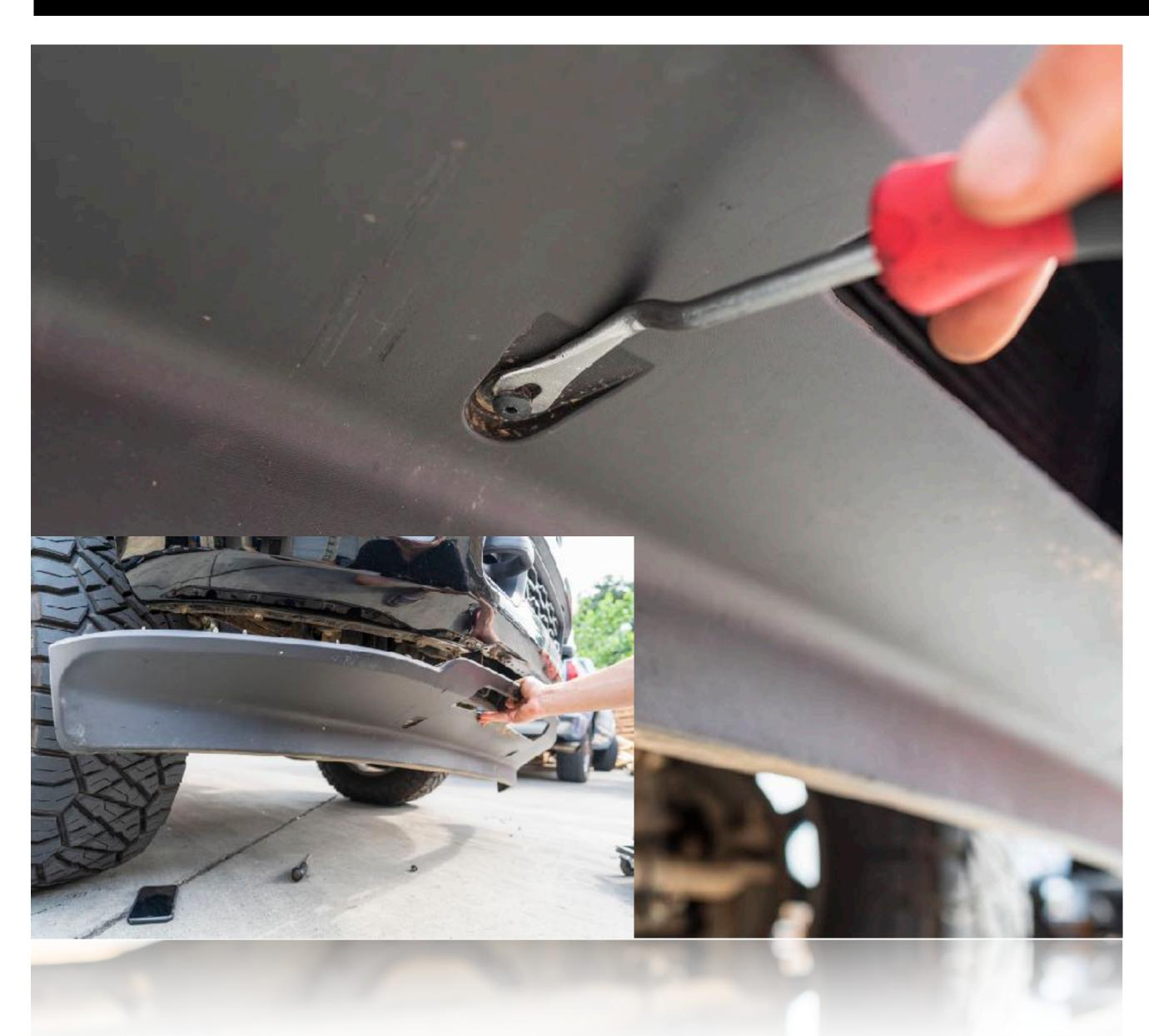
Undo the bolts on either side of the sunken center section of the bumper. Save the bolts for the next step.
