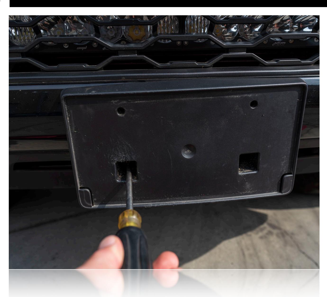
Remove the license plate bracket/mount with a flathead screwdriver.
