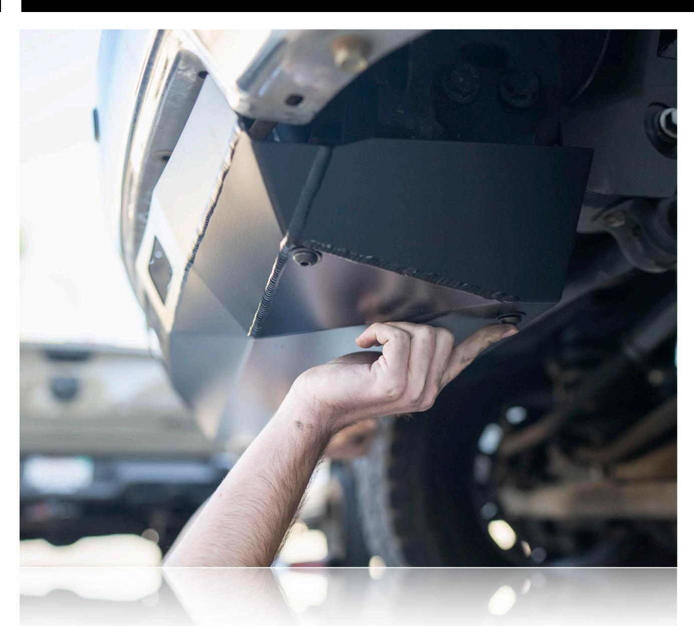
Access is tight, but we found it easiest to reach around from the side or front to hold the nut in place while tightening the skid plate onto the frame bracket.
