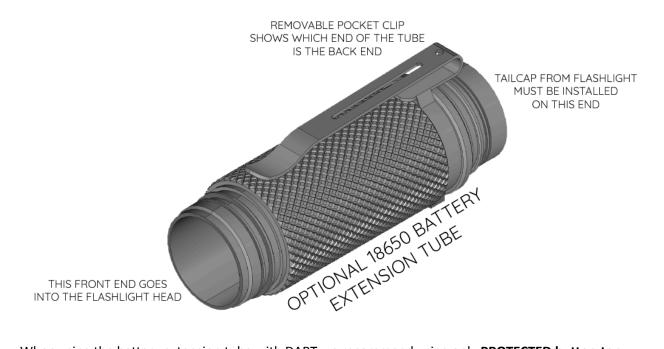
When using the battery extension tube with DART we recommend using only **PROTECTED button-top 18650 batteries made with trusted brand cells such as Panasonic, Sanyo, and/or LG.** Failure to do so may void warranty. Note: The body tubes can only work in one direction. If you find that your flashlight is not working with the tube attached, it is most likely backwards. Turn it around and try again.
