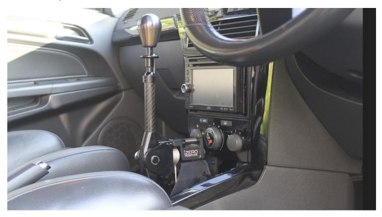
6 – Once all fasteners have been installed into the console and the Shifter correctly adjusted (see next pages), it's time to take it for a test drive and enjoy the ZPO Shifter! After the first outing, check that the grub screws have not moved (vibrations from the car can cause this). If they are moving too much, we recommend the smallest amount of blue/medium Loctite on them to counteract any vibrational movements.
