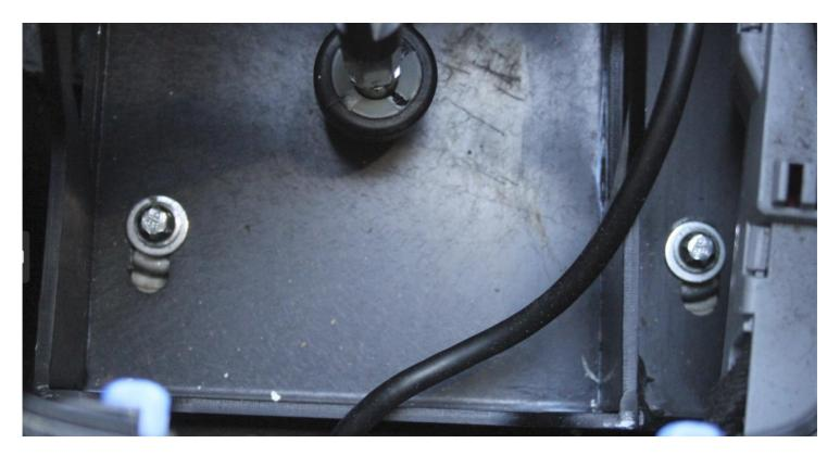
3 – With the Cables inserted correctly, the bolts can now be placed through the ZPO shifter mounting holes and tightened to secure the shifter into position.
