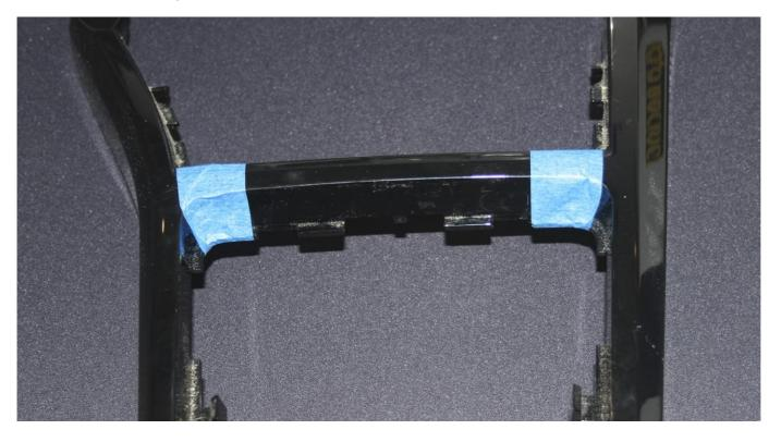
4 – If you are looking to run a centre console with the ZPO Shifter, you'll need to make some cuts using a Dremel or grinder (please use appropriate safety equipment) in the centre console and top cover. We marked ours with masking tape before cutting. As the VXR console is not symmetrical, you may want to line the cover up with the shifter before making marks for cutting.
