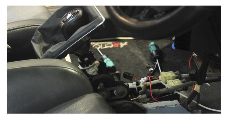
2 – Once removed, you'll have access to the OEM shifter, cables and mounting bolts. Remove the cables with the shifter in position for better leverage. Then remove the 4 bolts and the OEM shifter can be removed from the car. The ZeroPointOne Shifter can now be put loosely into position, fitting the cables into the mounting holes and the cable ends onto the ball studs.
