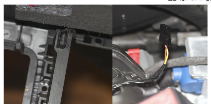
5 – Key Point! When removing the console, be aware that there are two electrical connectors that create a circuit for the wireless start/entry. Make sure these are re-connected.
