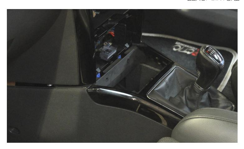
1 – The first step is to gain access to the OEM shifter by removing the centre console. There are several interior screws that need removing to allow the console to lift out. We also removed the radio head unit to gain access to some of these fasteners. The leather gearstick gaiter and leather handbrake gaiter will need to be prized from the centre console using an interior trim tool.
