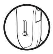
(2) Pull down the bracket, let the screw hole align the indicator arrow.
