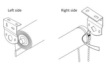
Install the tension device about 1" away from the shade and position it out of the reach of children. Extend the chain cord fully downward and mount it on the wall.
