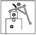
Snap the valance clips @ onto the headrail A.
