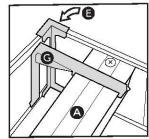
Snap the valance clips G near the edges of the track, while placing one valance @ clip on the center of the track.
