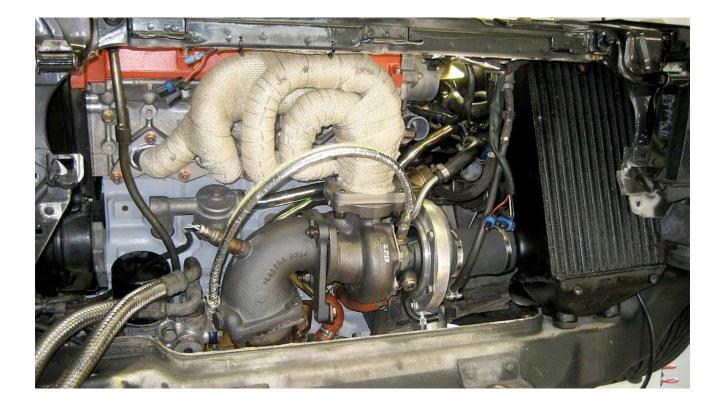
The picture shows a modified Lancia Delta EVO II with the plug'n'play ball bearing GT31SS wich has being customized to be used on Lancia Delta Integrale engines. This turbo is good for power outputs in the 350 hp range. Spool up starts already at 1700-1800 RPM and 0.5 Bar are reached at 2400-2500 RPM on a stock engine.
