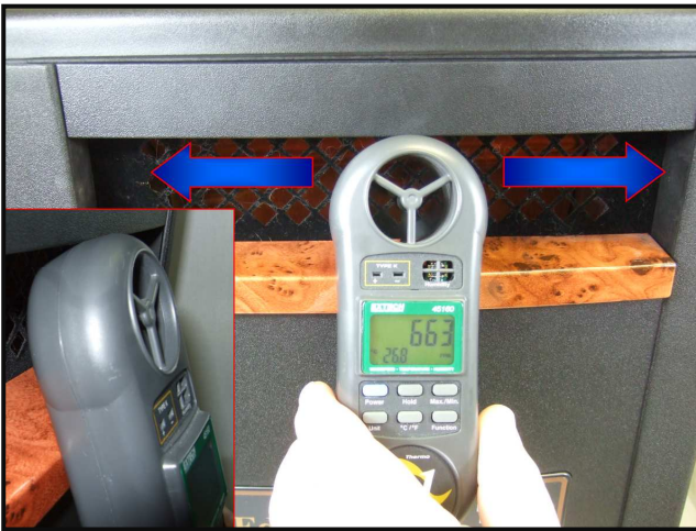
(FIGURE A) AIRFLOW TESTING
