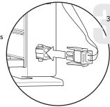
3. Insert the PCO cell connector into the plug on the plate cage. Press the connector firmly until the two tabs lock into place.
