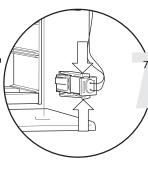
Unlock the PCO Cell connector by pressing on the connector's locking tabs.
