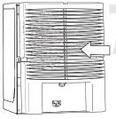
7. Replace the back cover by snapping into place.
