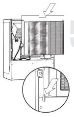
5. Replace the rear lint screen, inserting the bottom of the lint screen first.
