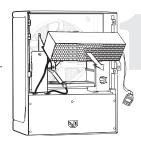
10. Slide the PCO Cell down and out of unit.
