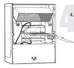
4. Gently insert the purifier plate between the guides (inside the cage) until it stops.
