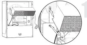
1.Slide the PCO cell up and into the unit. Be sure the back lip of the PCO cell engages the two slotted protrusions at the rear of the plate cage, and that the angle brackets and studs are correctly aligned.
