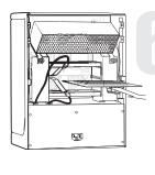
6. To remove the purification plate, grasp edge of plate in the center and gently pull out.
