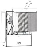
5. Remove the lint screen by pulling back the top, then lifting up and out.
