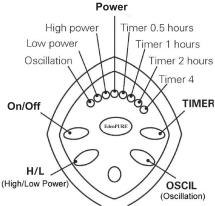
Temperature control: Press the H/L button to set the heating mode:
