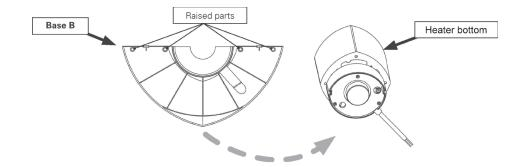
2. When assembling the EdenPURE All Season Infrared Heater, insert the four raised parts of Base B into the corresponding holes of Base A. There are two joints on Base B. Base B must be inserted into Base A until the sound that the two parts have been fitted together is heard.
