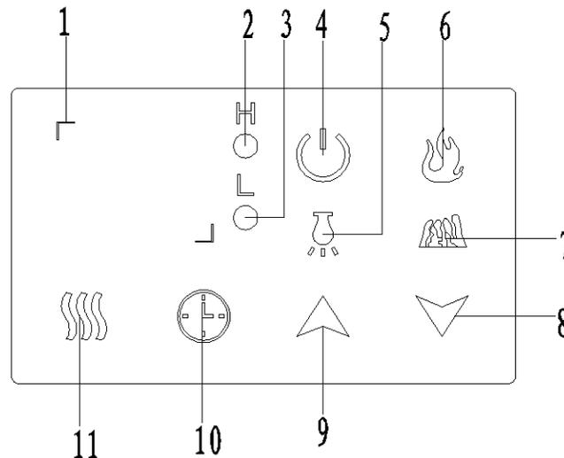
1. **Digital display:** Indicates the temperature that was set or the amount of time the unit will run.
