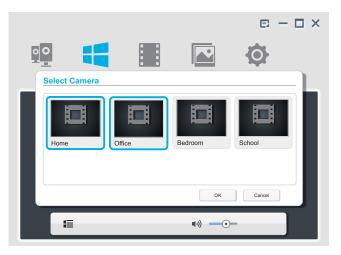
Select the right cameras from all the listed cameras, for Muliti-viewing on one screen. Select a camera preview to add it to the Muliti-viewing window, it will have a blue border. The blue border will disappear on clicking the camera preview again as it will remove the selection.
