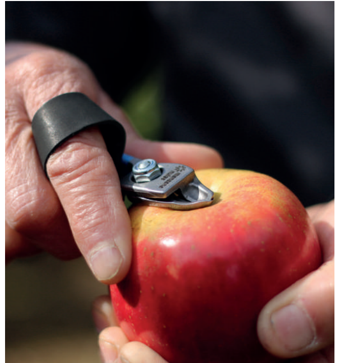
The concave shape of the blades adapts to the shape of the apple.
