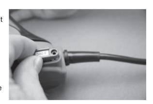
reattachment. B. Gently, using the "ears" on the module, pry the module evenly from the receptacle on the left handle. Please observe that the module's connection prongs are small, delicate and must be protected from damage.
