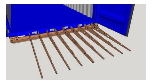
Position part G on edge (slots pointing down) over the corresponding slots of parts A and B.
