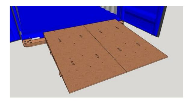
When you are happy with the assembly of the ramp and the deck position, fasten the decks to the framework using 4x40mm wood screws, tightening them flush to the surface through the holes in the deck surface (50 in total) You may also wish to use a small amount of wood glue between the A/B framework and the ramp surface.
