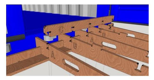
Adjust A and B positions where necessary so that C slots into all five pieces, locking them all together.
