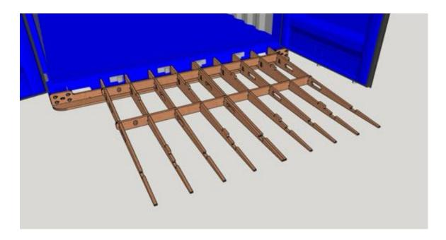
With part H flat, line it up over the remaining slots in the A/B frame.
