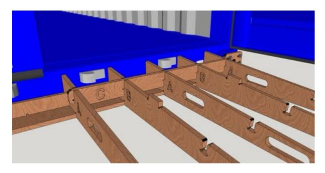
Slot the remaining part C into the corresponding slots...
