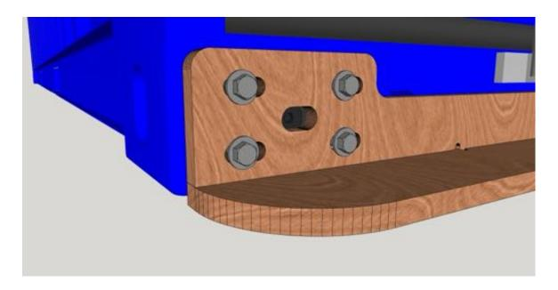
Attach the right hand side of E/F to the other Domino Clamp. When all the screws are in position, tighten each one firmly.
