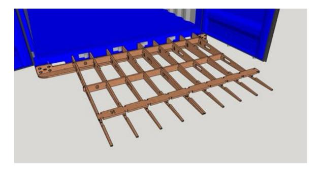
Push it into position completing the support frame for the 1800mm wide double ramp.
