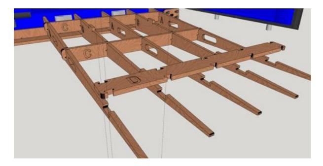
Drop it into position completing the support frame for the 900mm wide single ramp.
