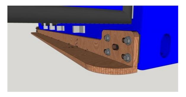
Position one of the Part A sections over E/F just to the right of the centre of the container.
