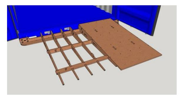
Line up the 4 protruding tabs on parts B of the right hand framework with the holes in one of the ramp decks until it sits flush to the ramp framework.
