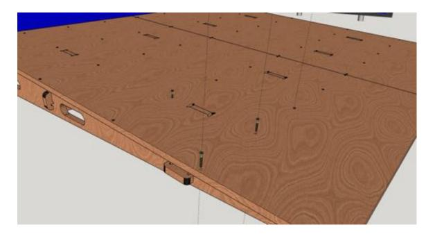
We suggest finishing the ramp (especially the E/F bracket) with a couple of coats of polyurethane varnish, watered down PVA, or similar protective finish.
