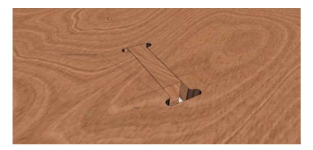
If needed, a small amount of adjustment can be made to the ramp surface's position so it can be slid flush to the doorway's edge.
