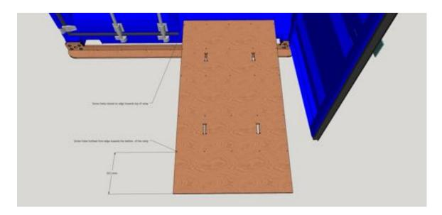
Line up the four protruding tabs on parts B with the holes in the ramp surface...
