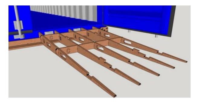
With part D flat, line it up over the remaining slots in the A/B frame.
