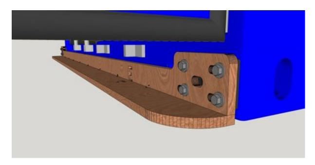
Slot one of the Part A pieces onto E/F near the left hand side of the door opening.
