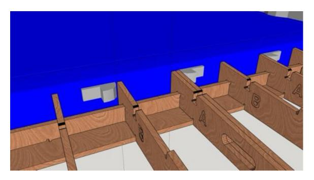
Add alternating B/A parts mirroring the first set of A/Bs, and their spacing.
