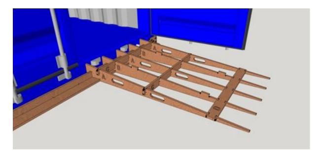
Line up the ramp surface so the line of screw holes close to the edge are at the  $\underline{top}$  of the ramp.
