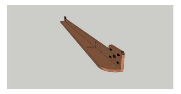
Using 4x40mm wood screws join parts E and F through the holes behind and underneath.
