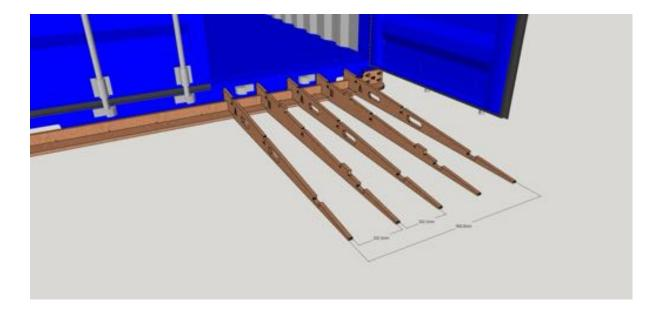
Position part C (slots pointing down) over the corresponding slots of parts A and B.
