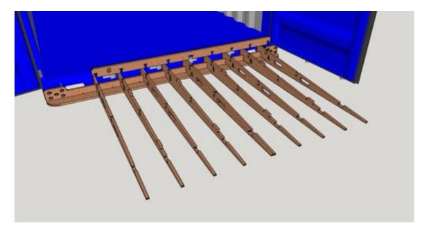
Adjust A and B positions where necessary so that G drops down, locking them all together.
