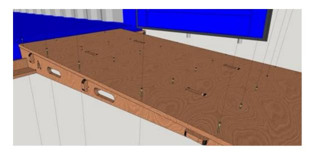
You may also wish to use a small amount of wood glue between the A/B framework and the ramp surface.
