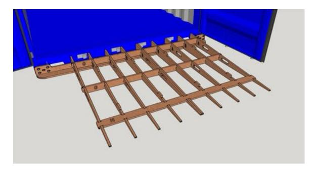
Line up the ramp surface so the line of screw holes close to the edge are at the  $\underline{top}$  of the ramp.
