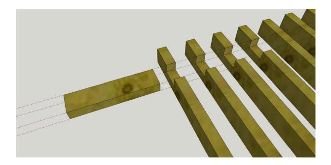
12. From the door end of both rails, mark every 610mm and place a stud centered over each mark and fix them into place. The last being placed against the end stud.
