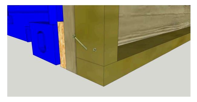
11. Take ten studs and make a notch the width and depth of your 4"x2" timber 2350mm from one end.
