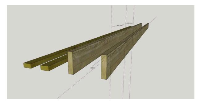
5. Join the 4"x2" timber on edge to the 8"x2" using 90mm screws to form an L. These will form the top and bottom rails for your studs to fit to while providing a strong straight edge to span between the Domino Clamps.
