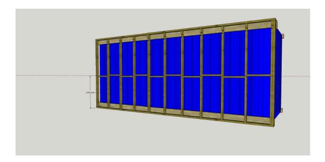
14. Cut a piece of 4"x2" to fit between the end studs, place on edge into the channel formed by the notches at the top of the intermediate studs and fix it through the face and ends.
