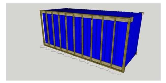
13. Next, cut noggins\* to fit in between each stud and fix them approx 1220mm up from the lower edge of the bottom rail. It helps to stagger their position to make fixing through each stud easier.
