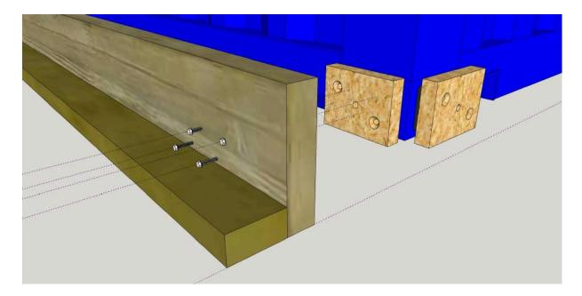
8. Repeat this previous step for the top rail. It should be flush with the roof of the container, the 4"x2" is on the top edge and both rails are plumb and parallel to each other.
