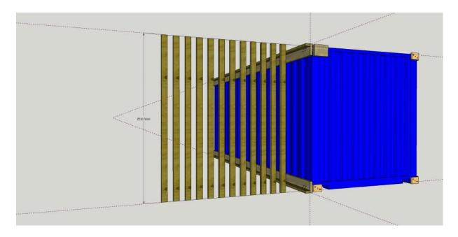
10. Place one stud flush at each end of the rails, secure into position using screws or nails diagonally through the stud into the rail.
