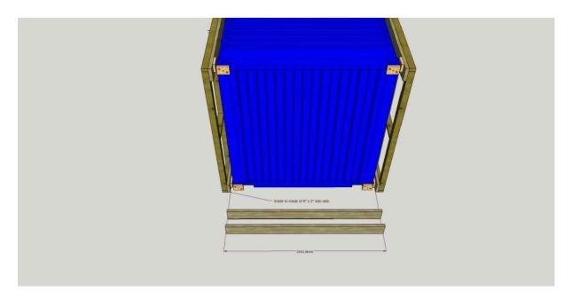
16. Next, measure the horizontal distance from the outer edges of the 4"x2" rails and cut 2 lengths of 4"x2"
