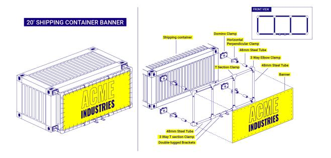
Creates an rectangular frame with an internal aperture of 2.45m(h) x 5.8m(w)
