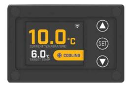
Use the 'up/down' buttons to change the target temperature. Hold the 'set' button to pause or resume the cooling and/or heating signal. This may be useful when transferring your beer out of the fermenter. To enter the controller settings press the 'set' button, then navigate using the 'up/down' buttons and press the 'set' button to select an option.
