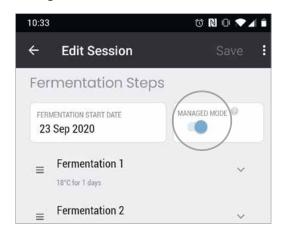
9. The Conical Fermenter Pro Controller, in conjunction with the Cooling Pump Kit/Glycol Chiller, will now automatically maintain and change the fermentation temperature based on your profile. Under fermentation tracking, you can view a graph that monitors the progress of your fermentation.
