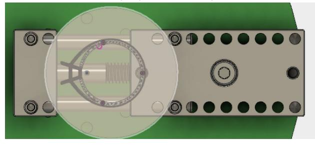
Finally, the moveable jaw is adjusted back to the right so that the grippers on the moveable jaw overlap the stock in the same way at the grippers on the fixed jaw.
