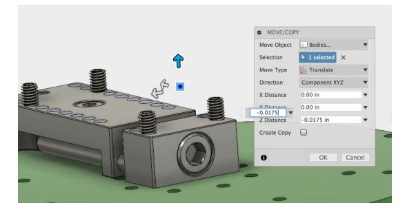
Enter the amount by which the B-table offset in the model needs to be adjusted in order to match the machine's offset. Click "ok" to apply the change. It is good practice to verify the new location has updated properly before saving the file. Note that the offset will only need to be adjusted in Z direction. It should never be moved in the X or Y axes. Make sure to save the file before proceeding.
