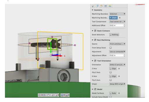
The heights are set up as shown below. The bottom plane is coincident with the back of the gem setting and top plane is 0.1 inches inside the stock surface. In most cases the top plane must lie outside of the stock surface, but since the material has been removed already it is more efficient to let the tool rapid feed closer to the cutting depth.
