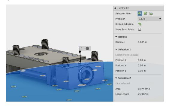
The B-Table Offset, is the point in space about which both the A and B tables rotate. This point in the model must match the point in reality in order for the part to be oriented correctly relative to the machine when the rotary axes are moved.
