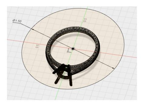
Next, select the circle just created and extrude it both directions. Extrude one side 0.3 inches and the other side 0.7 inches. Change the opacity of the body created by the extrude to30% so that the ring is still visible inside of it. The goal of this step is to locate
