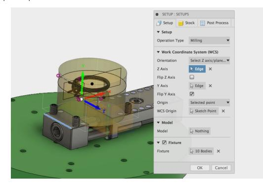
This orientation corresponds to the way the axes are aligned when the machine is the its home position. The B table is flat or parallel to the spindle of the Pocket NC mill in the home position. The Y axis moves the table up and down. The Z axis is parallel to the spindle and the X axis is perpendicular to both Y and Z and moves the A and B tables forward and back. The home position of the machine is shown below for reference. The spindle is to the top of the image.
