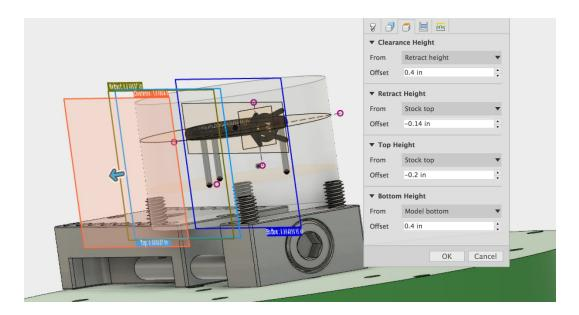
The tool pass settings are shown below. Note that the tolerance is the same as the one on previous two operations and the tighter than the ones used for the clearing
