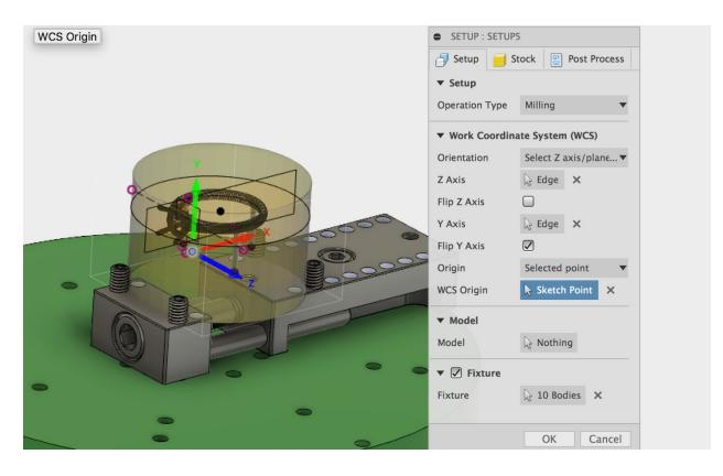
The "Model" tab is left with no selection. The model will be defined for each machining step instead.
