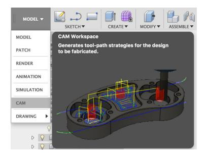
Before any toolpaths can be created a setup has to be created that defines the location of the origin, the stock, the fixtures, and the coordinate system. These features must be chosen in a way that makes it possible to make the physical setup on the machine match the one used to write the toolpaths in the model. To create a Setup select the setup dropdown and "New Setup".
