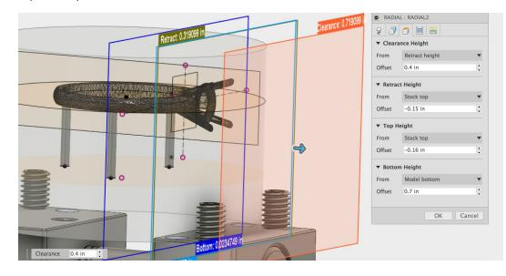
The tool pass settings are shown below. Note that the tolerance is the same as the one on the previous three operations and tighter than the ones used for the clearing operations. The stepover is very small in order to produce a good surface finish and the level of detail desired. If the finished product is rougher than desired this value may be further reduced at the expense of a larger file size and longer machining time.
