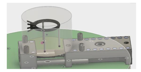
Next, the stock is moved back to the right so that it just barely overlaps the grippers on the fixed jaw. This overlap is to account for the crushing/biting into of the stock material that occurs when the vise is closed. The overlap should be about 0.01in. This overlap
