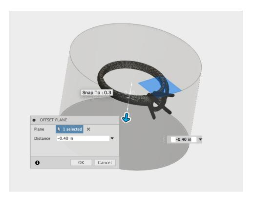
Sketch three center-diameter circles on that new offset plane by selecting points around the perimeter of the ring that are spaced fairly evenly as shown below. Do not place any supports close to the front of the ring. These will be supports left in place during the machining and would interfere with the machining of the prongs if they were placed in the front.
