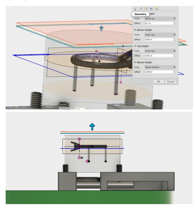
The tool pass settings are shown below. Note that the tolerance is tighter than it has been for previous operations. The pass direction controls the way which the ring is cut. The settings shown will start at the tips of the prongs and work back toward the ring. This is desirable because it means there is more material on the prongs to support the cutting forces when the tips are being milled. Cutting the opposite direction runs a greater risk of breaking the the prongs off.
