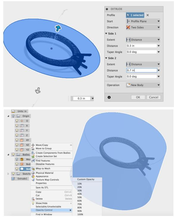
The ring has to be supported while it is being machined so that is maintains its position in space and can be reliably located. In order to avoid cutting away all of the support structure, geometry that will be avoided by the machining process is created.
