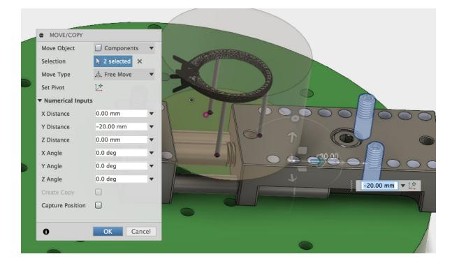
The grippers on the fixed jaw(the one with two rows of 9 holes drilled in it) are moved 20mm to the left. The holes are 5mm apart so the grippers are moved 4 holes to the left. Since the grippers must fit in the holes the adjustment of the fixed jaw is in 5mm increments.
