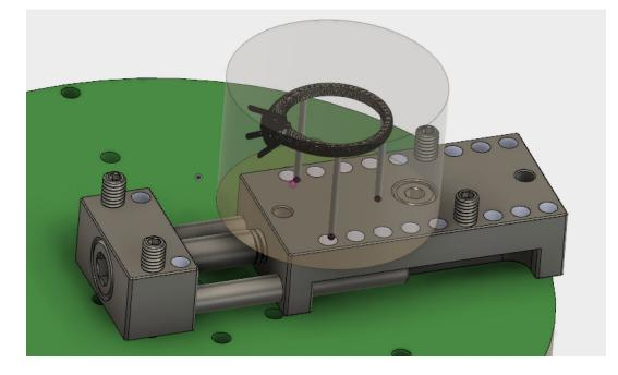
The workpiece is then moved about 20 mm to the left as well so that the grippers on the fixed jaw can be more easily accessed.
