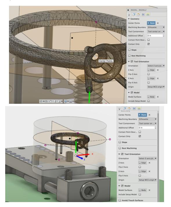
Next, the heights are set as shown below. Both the top height and the retract height are set to be within the stock envelope because the material in that area has been removed so collisions will not take place.
