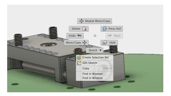
When the dialog box opens, change the selection filter to "Bodies." Select the origin as the body to be moved. Calculate the distance that the origin needs to be moved. In this
