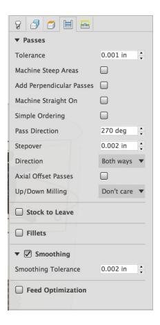
The linking settings are the final settings to adjust before generating and simulating the toolpath. All of the settings below should be the defaults.
