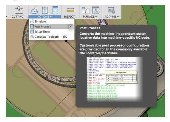
While the ring may be saved as one program file, it is recommended to use as separate program for each tool. For the ring, this will mean two programs; one for the first three operations with the  $\frac{1}{8}$  inch end mill and another program for the last 5 operations done with the 1/32 inch end mill.
