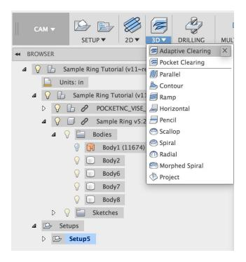
A dialog box will open where the parameters for the toolpath are entered. The first parameter to be set is the tool. Click on the "Select" button under the tool tab. This allows a tool to be chosen from the tool library. Scroll all the way to the bottom of the list of tools and select tool 6, ½ inch flat 45 deg. end mill, out of the "Local Library" which is the Pocket NC tool library.
