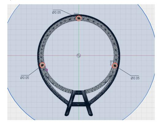
Extrude the circles up to the bottom of the ring to form the supports. Make sure that the operation chosen is "New Body."
