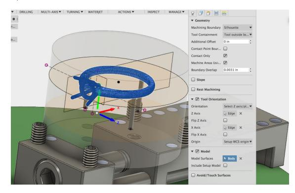
The heights are set as shown. Both the top height and the retract height are set to be within the stock envelope because the material in that area has been removed so collisions will not take place.
