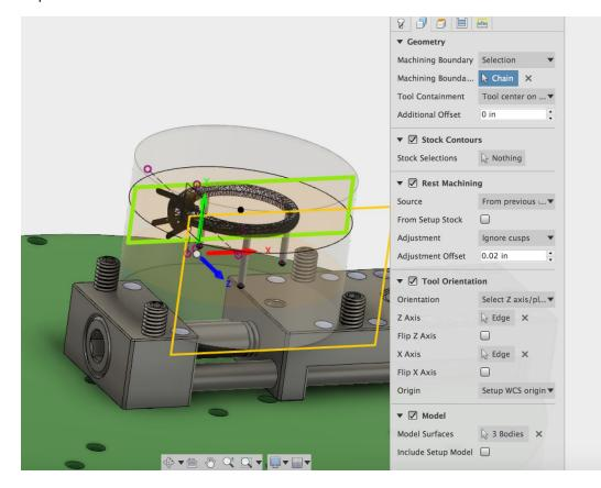
Set up the heights as shown. The bottom is coplanar with the midline of the ring. It is referenced from the world coordinate system origin.
