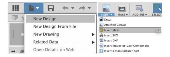
.stl files exist in two formats, English and Metric format. If the geometry is imported using the wrong format, the sizing will be much larger or smaller than expected. Import the Sample Ring using **Metric units**. Using the Inspect icon, users can measure the distance between prongs and check for a correct import.
