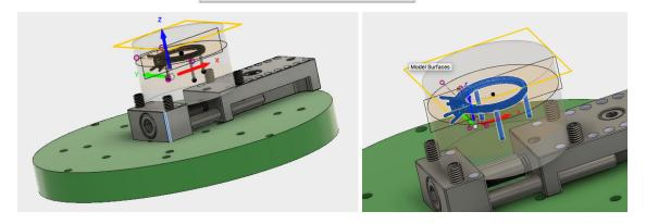
Next, select the "Heights" tab to set the top, bottom, retract and clearance heights. These heights define the space in which the tool is allowed to operate. The retract plane defines the height to which the tool is retracted during drilling or pocketing operations. The clearance plane is the height to which the tool must be retracted before rapid movements or rotation of the tables is allowed. These planes must be selected appropriately so that collisions are avoided.
