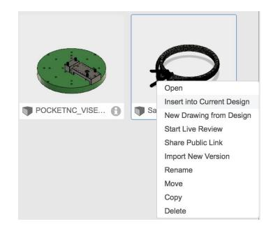
The part will not usually import in the desired position. The first step in the setup is to used the the move commands locate the part in approximately the desired location and orientation.
