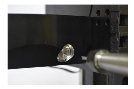
The tool will advance until it triggers the tool probe button. It will then retract a short distance, and then approach at a lower speed until the button triggers again.
