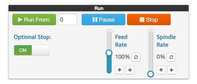
If you have a M0 or M1 command at the start of your code, the program will be paused. Click the blue Pause/Resume" button or push the green Pause/Go button on the machine in order to start the program. The user may pause the program at any point by clicking the "Pause" button or pushing the green button on the machine. The user can stop the program by clicking the "Stop" button or pushing the red, emergency stop button on the machine.
