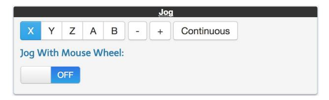
The user can also jog the axes using the mouse wheel by turning enabling the "Jog With Mouse Wheel" button and selecting the desired axis of motion by clicking on the respective button.
