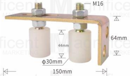
Upper Guide Bracket #80 Guide – Php889/pc Roller Material: Nylon Roller Diameter: D30mm Size: 64mm x150mm
