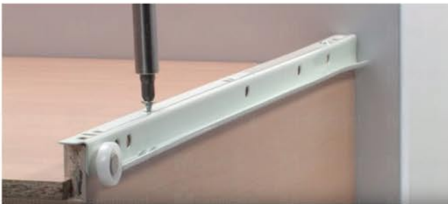
INSTALL THE RUNNER UNDERNEATH THE DRAWER fasten the drawers with screws with holes as a guide
