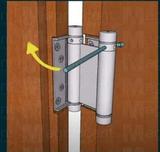
4. ADJUST THE RESILIENCE Stick the adjusting bar to the adjusting hole to adjust the hole position and then insert the pin to fix the position (Different holes represent different resilience)
