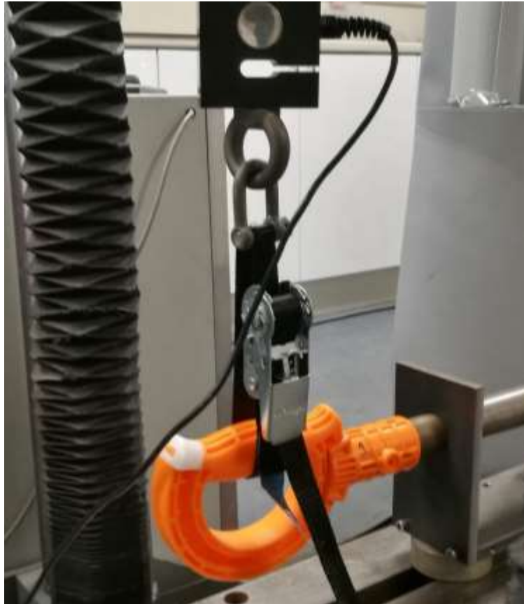
Image 2: Test setup showing vertical loading
