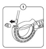
If the track on the handles becomes clogged up with debris, simply pop off the track closure cap to clean
