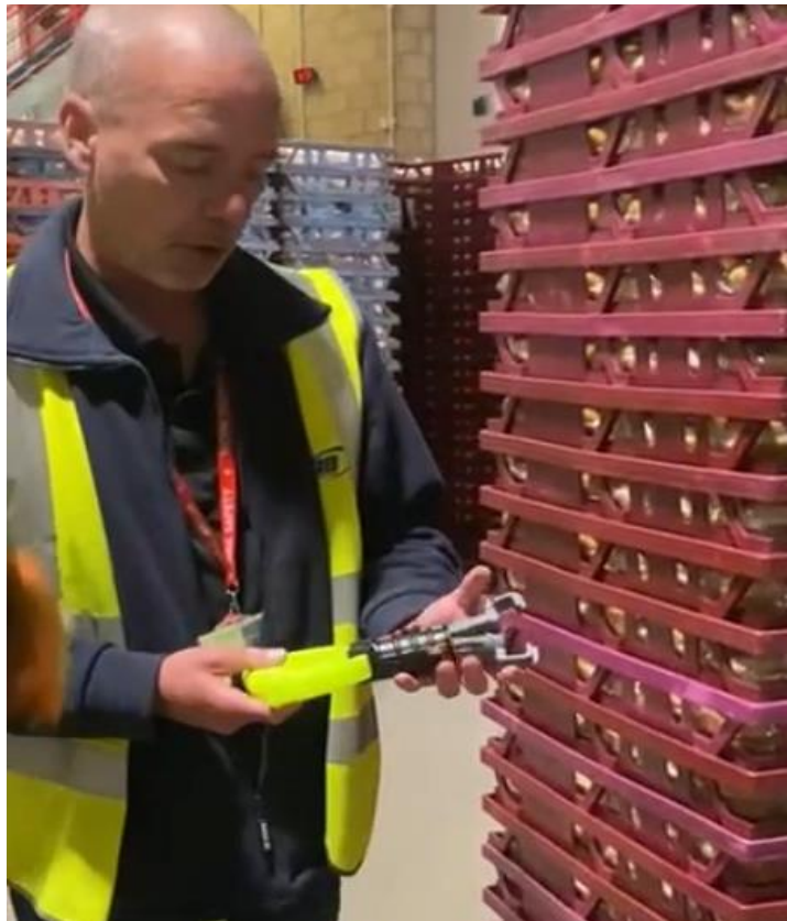
A bespoke Safety Handle for a burger bun rack
