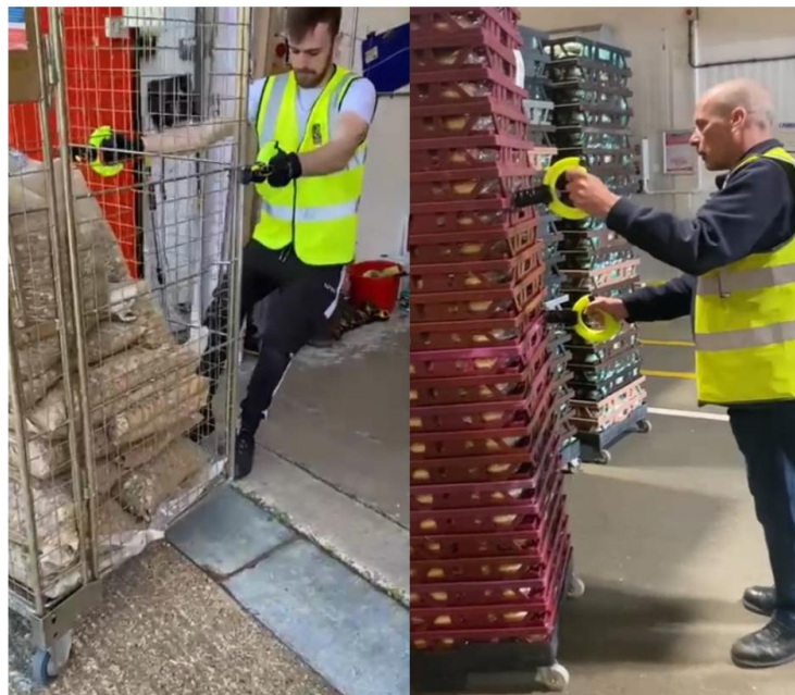
iRoll Safety Handles providing safety with 500Kg loads and unstable bun tray towers
