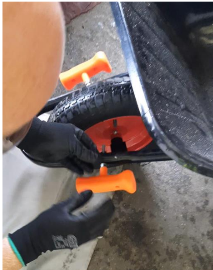
Fitting ezTip Safety Handles to the nose of the wheelbarrow
