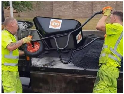
A <u>2 person Safety Handle set</u> reduces the chance of losing grip as well as back and wrist injury during "muck away" lifting requirements.
