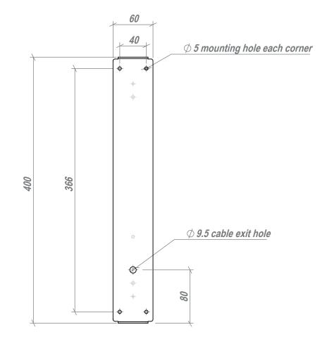
Backplates can be rotated 180 degrees- to allow cable exit to be positioned at top if required.
