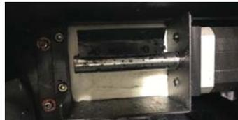
Clean the capping station seal with alcohol and a lint free swab until clean. Inspect capping station seal for any cuts, tears or other signs of wear. Replace if the seal can no longer create an airtight seal with the print head.
