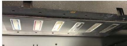
Inspect the bottom of the UV lamp. If the lens has ink on it, clean with UV cleaning solution or alcohol until the lens is completely clear. If using UV cleaning solution, use alcohol after to remove any cleaning solution residue.
