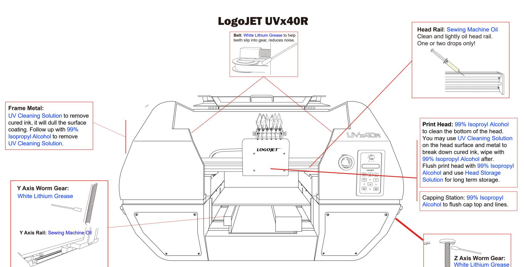
UV Cleaning Solution - Use for cured ink on metals. Clean off residue with 99% Isopropyl Alcohol.
