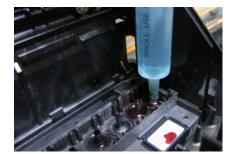
Once all the ink is flushed from the head, you must then clear the solution from the nozzles by flushing with air. Fill the syringe with air, place on the post and push the air through the nozzles.
