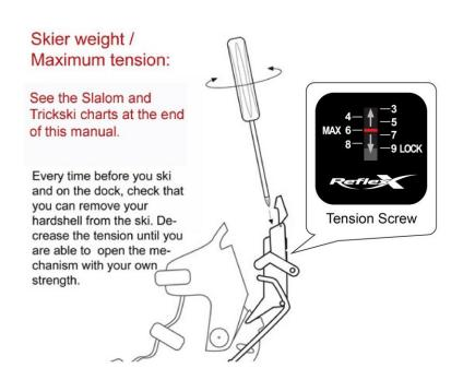
The release mechanism must be set in accordance to the weight and the skiing style of skier.
