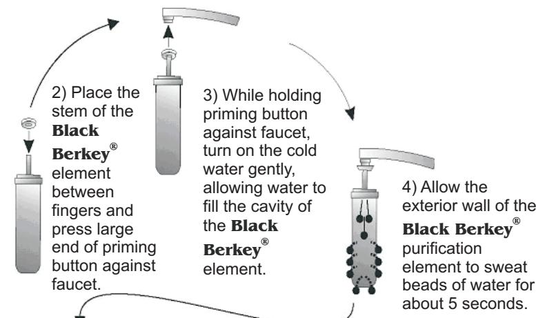
5) Rinse process dust from exterior of purification element. The element has now been successfully primed. Repeat steps 1 - 5 for each additional element.
