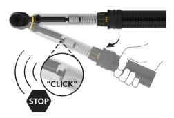
**3.** Wrench will automatically reset for next operation after pressure is released.
