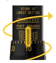
**4.** Lock the torque setting by turning the locking knob clockwise until snug. Wrench is now set to measure 130 ft.-lb. of torque and ready to use.
