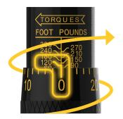
**3.** The micrometer scale divides the main scale into 15 divisions, each marking representing 2 ft.-lb.
