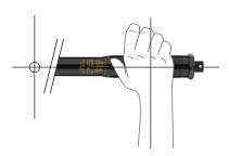
2. Operate the wrench to tighten the nut/bolt, gradually increasing the force until they are snug. Slow down your operation and apply a smooth and steady pull. When you hear or feel a 'CLICK' or 'IMPULSE', stop pulling the wrench and release the pressure on the handle.
