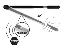
**3.** The wrench will automatically reset for the next operation after pressure is released.
