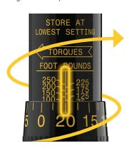
**4.** Lock the torque setting by turning the locking knob clockwise until snug. Wrench is now set to measure 120 ft.-lb. of torque and ready to use.
