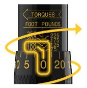
3. The micrometer scale divides the main scale into 10 divisions, each marking representing 2.5 ft.-lb.
