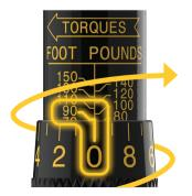
**3.** The micrometer scale divides the main scale into 10 divisions, each marking representing 1 ft.-lb. To adjust the torque from 90 to 95 ft.-lb., rotate the micrometer handle in a clockwise direction until the "5" mark (5 micro-movements) aligns with the vertical line on the main scale. This adds 5 ft.-lb. to the main scale reading of 90 ft.-lb., resulting in a total torque of 95 ft.-lb.
