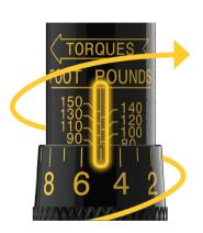
**4.** Lock the torque setting by turning the locking knob clockwise until snug. Wrench is now set to measure 95 ft.-lb. of torque and ready to use.
