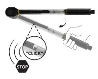
**3.** The wrench will automatically reset for the next operation after pressure is released.
