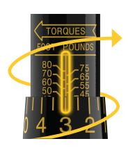
4. Lock the torque setting by turning the locking knob clockwise until snug. Wrench is now set to measure 53 ft.-lb. of torque and ready to use.
