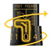
**3.** The micrometer scale divides the main scale into 10 divisions, each marking representing 0.5 ft.-lb.
