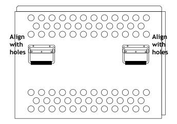
NOTE: IT IS IMPORTANT TO HAND ASSEMBLE ALL NUTS AND **BOLTS BEFORE FINAL TIGHTENING.** Attach back panel(B) to base panel(A) using (3) machine screws and nuts. Do not tighten nuts and bolts until the crate is assembled completely.
