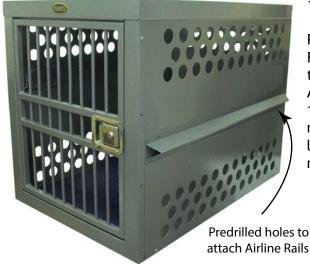
Position the AIRLINE RAILS to match up with the predrilled holes. Assemble using (16) 10-32 x 1/2" Pan Head machine screws and lock nuts (included with rails).
