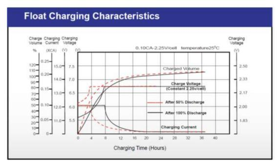
80 % capacity ~ up to 6 to 9 hours charging time depending on the discharge level.
