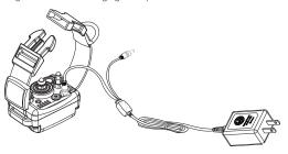
Indicator light will turn solid red during charge cycles and will turn green once it is fully charged. (approximately 2 hours)
