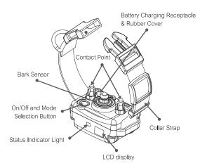
The BP-504 is outfitted with a waterproof control button which is used to turn the unit on and off, toggle through the five modes, and change the settings of the different modes.
