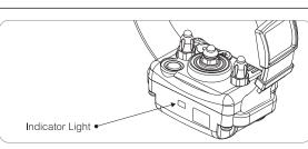
Once the unit is turned on the indicator light will flash green when the battery is charged. It will flash amber when it needs a charge within the next 24 hours and red when charging is required for continued operation. The BP-504 will go into a sleep mode if there is no programming or bark activity. In sleep mode the unit will still detect barks but will not show the battery life, simply pressing the control button will wake up the unit.
